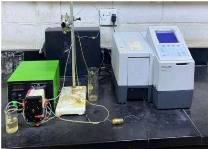
Fig. (3.3) : Flow Injection System With Uv-Vis Detector.
